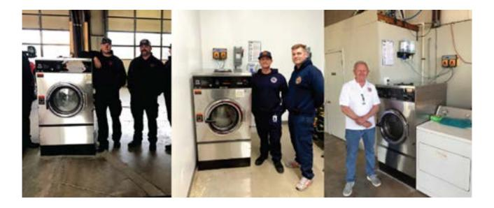
Specific laundry equipment, such as the Dexter 100 G Series Washers and the Circul Air Express PPE drying cabinet, works by removing pathogens from your crew's gear. They are designed with industry-specific cycles, temperature recording, and fire response systems. These units decontaminate your equipment while curtailing damage and the life of the gear.
